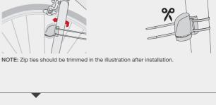
NOTE: Sensor uses A23 12V battery.
