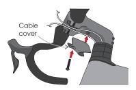
Make sure the cables are inside the cable cover.
