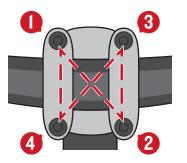
Make sure the gap is equal on the top and bottom. If the spacing is unequal, loosen the bolts and retighten them following the order above.
