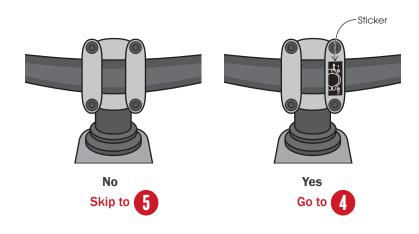
Tighten the top two faceplate bolts one half turn at a time — switching back and forth — until you hear the tool click. Then tighten the bottom two.
