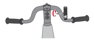
Loosen the faceplate bolts a few turns and rotate the handlebar up until it's the same angle as the forks or the brake levers are about 45° to the ground. Then tighten the faceplate bolts until they are snug.
