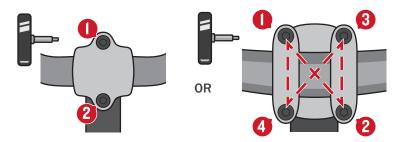
Make sure the gap is equal on the top and bottom. If the spacing is unequal, loosen the bolts and retighten them following the order above.
