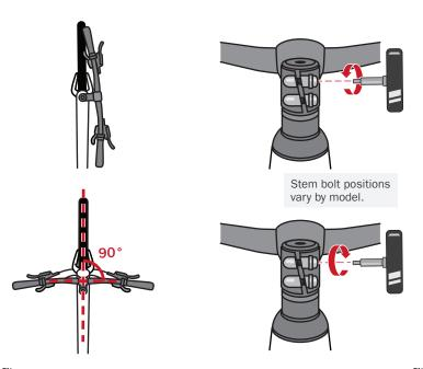
If the stem bolts look like this (see below), fully tighten the fasteners on the drive side of the barstem — switching between them — until they are fully torqued. Then fully tighten the fasteners on the non-drive side of the barstem — switching between them — until they are fully torqued.
