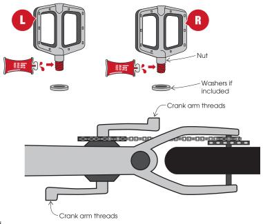
Thread the pedals in by hand — tightening by the nut, not the pedal. Then use the pedal wrench to fully tighten the pedals.
