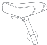
Figure 1.2: The seatpost minimum insertion line.
