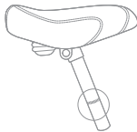
Figure 1.2: The seatpost minimum insertion line.
