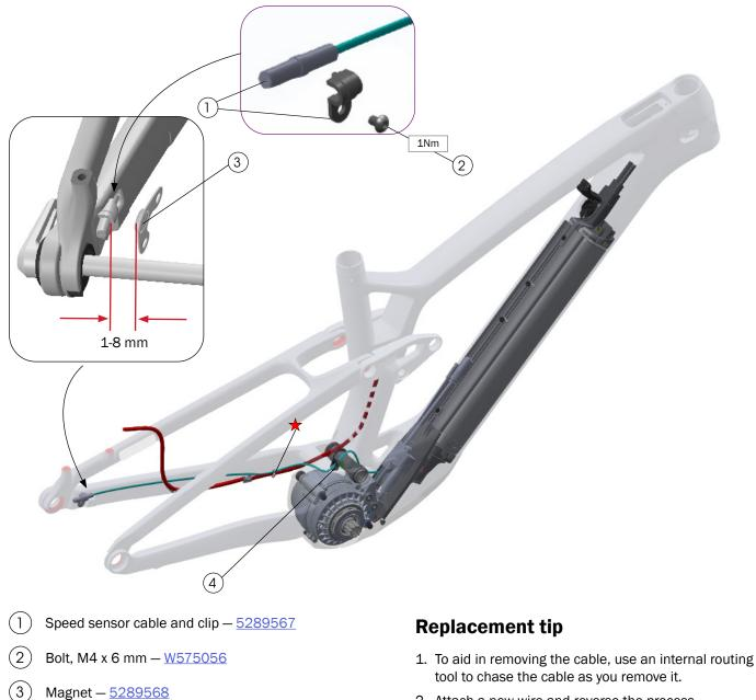
2. Attach a new wire and reverse the process.
