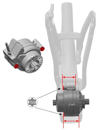
**NOTE:** Only adjust the compensation screws if you are replacing the drive unit.
