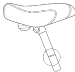
Figure 1.2: The seatpost minimum insertion line.
