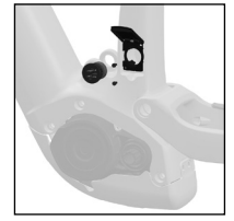
Battery charge port
