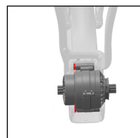
Adjust the compensation screws
