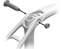
IsoSpeed: remove and install
