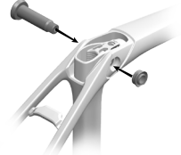
IsoSpeed: remove parts and install
