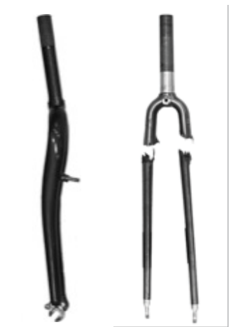
Figure 1. Overloaded forks: metal fork on left bent when overloaded. Carbon fibre fork on the right broke at a much higher load, but completely separated.
