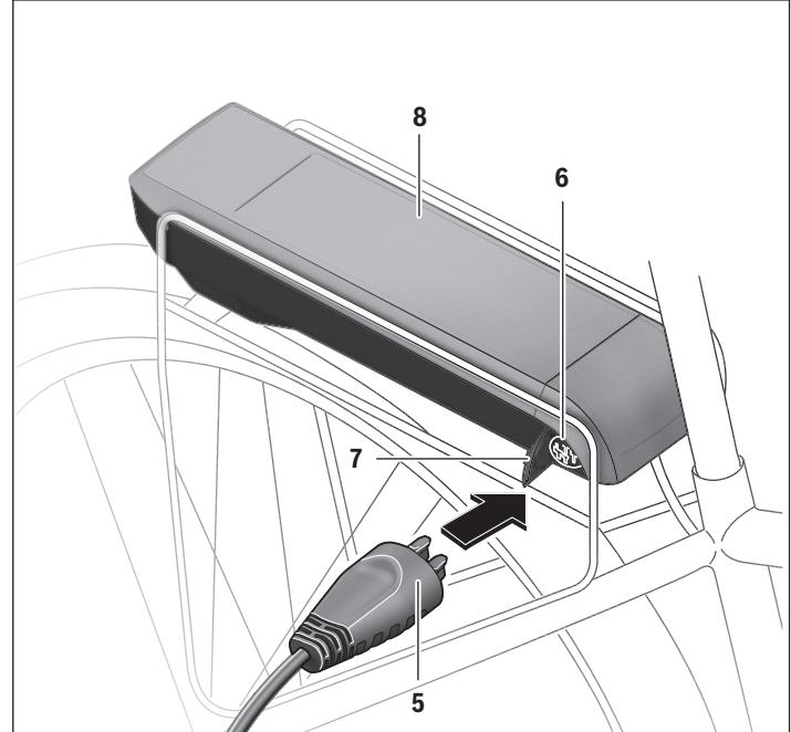
Switch the battery off. Clean the cover of the charge socket **7**. In particular, prevent the charge socket and the contacts from getting dirty, e.g., with sand or soil. Lift the cover of the charge socket **7** and plug the charge connector **5** into the charge socket **6**.
