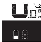
If an eBike has two battery packs being charged on the bike, the charging progress of both battery packs will be indicated on the display (the left-hand battery pack is being charged in the illustration). You can tell by the flashing indicator on the battery pack which of the two battery packs is being charged.
