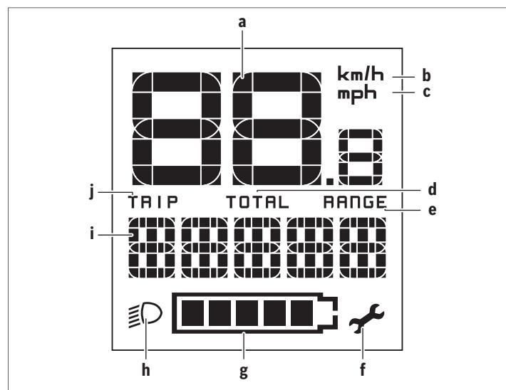
The **speed indicator a** always displays the current speed.
