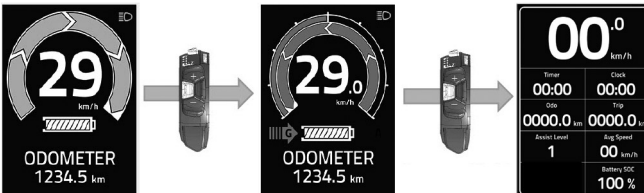
Simple screen - Left toggle (4 sec) - Enhanced screen - Left toggle (4 sec) - Technical screen
